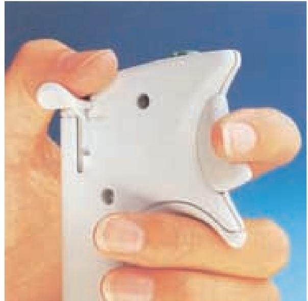
*By sliding the lever around the top of the handle, the soft-touch tip ejector can be positioned for right- or left-handed use.*
