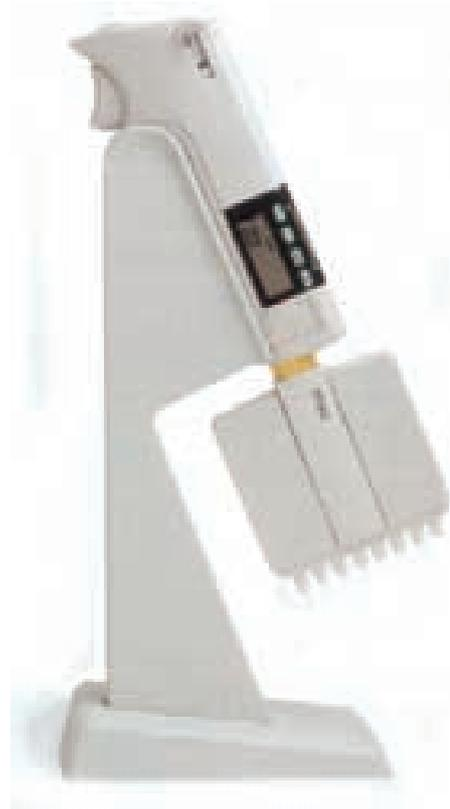
The BioControl recharge and storage stand has a rapid recharge (45-60 minutes) function. Overnight recharge is activated automatically when the Finnpipette BioControl is placed on the stand. The universal handle emits an audible recharge signal when the battery is going low, and a recharge message flashes on the display.
