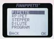
The intuitive menu displays the most commonly used functions, such as PIPETTE. Selecting PROGRAM accesses nine different user memory slots available for storing your own combinations of the 10 different pipetting functions.
